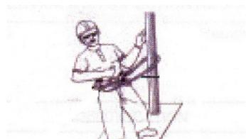
**Step 2:** Loop the lanyard twice around the structure and connect the other end to the other anchor point on the belt. Adjust the length of the lanyard using the adjuster.
